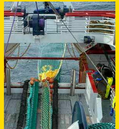
▲ Shooting away the single-rig hopper net during fishing trials off Thyboron last week.
